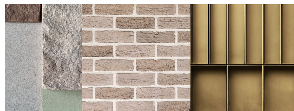
Materials being tested: Warm tones of local pink Doddington stone and brick, combined with gold coloured profiled metal panelling
