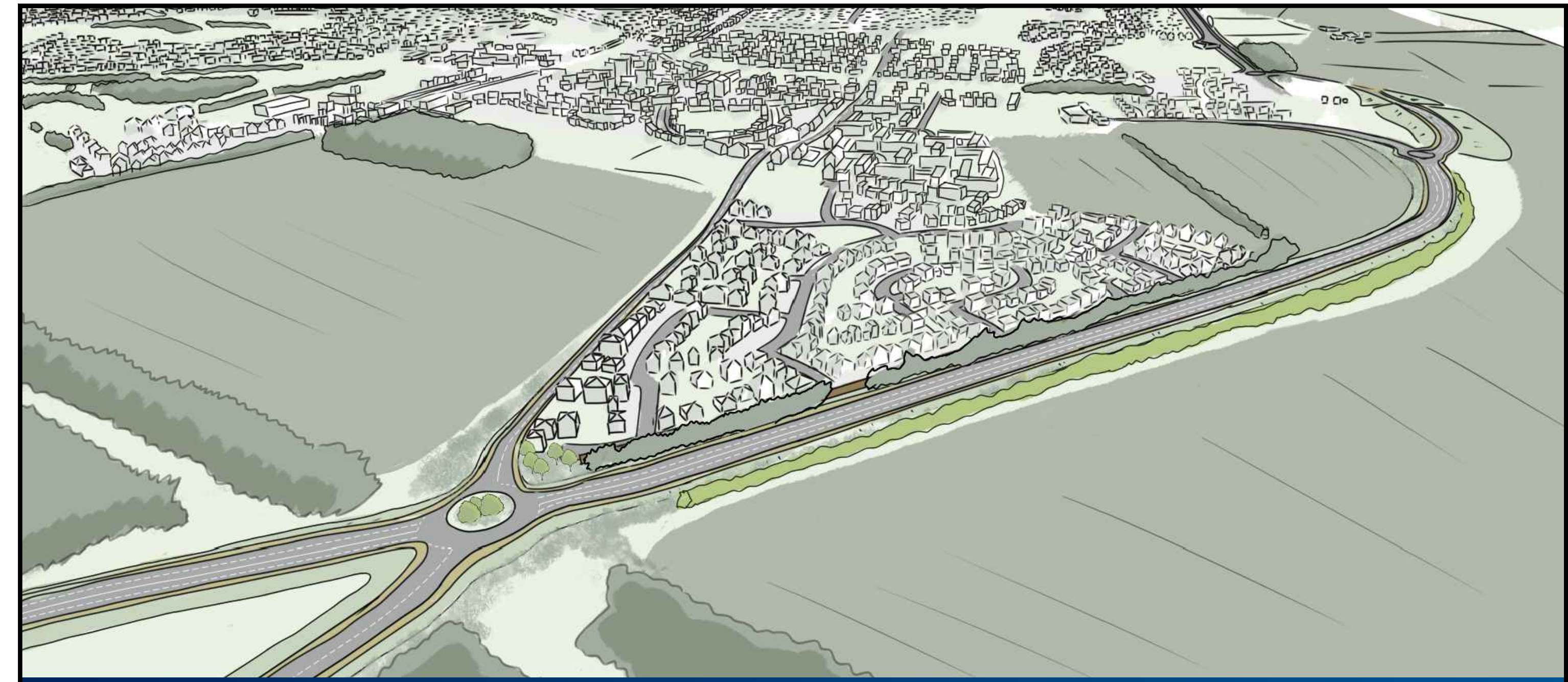
2 NORTH EAST VIEW Route of A1061 to be dualled & new roundabout in foreground at Portland Wynd
